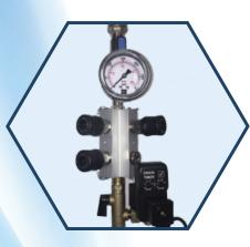
Complete drop assembly shown in vertical orientation with electronic timer drain, 90900-04, to remove condensate. This installation also features universal quick couplers and the gauge kit to monitor point of use air pressure.
