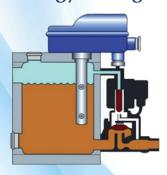
When condensate level reaches the high level sensor, the solenoid valve is activated and the condensate is discharged.
