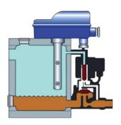
As the level of condensate reduces, it reaches the low level sensor, which signals the valve to close. NO AIR IS LOST!
